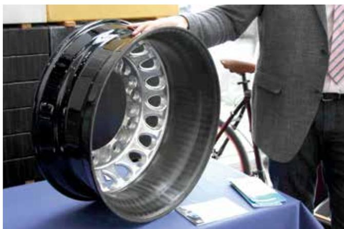
With the increasing importance of mobility comes a need to make sparing use of resources. A mix of materials is used for lightweight wheel rims.
