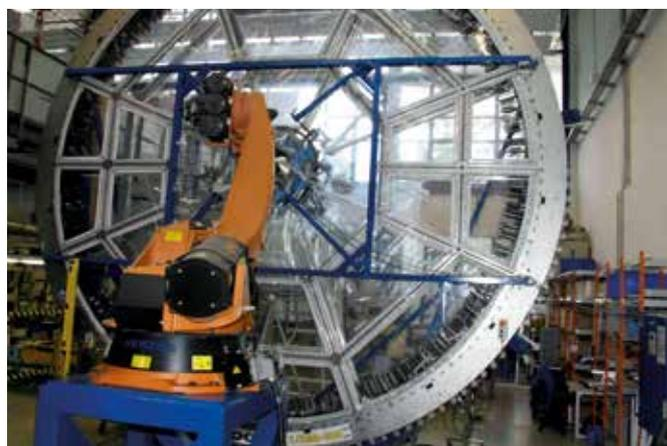
Automated weaving of carbon fibres makes lightweight structures possible.
