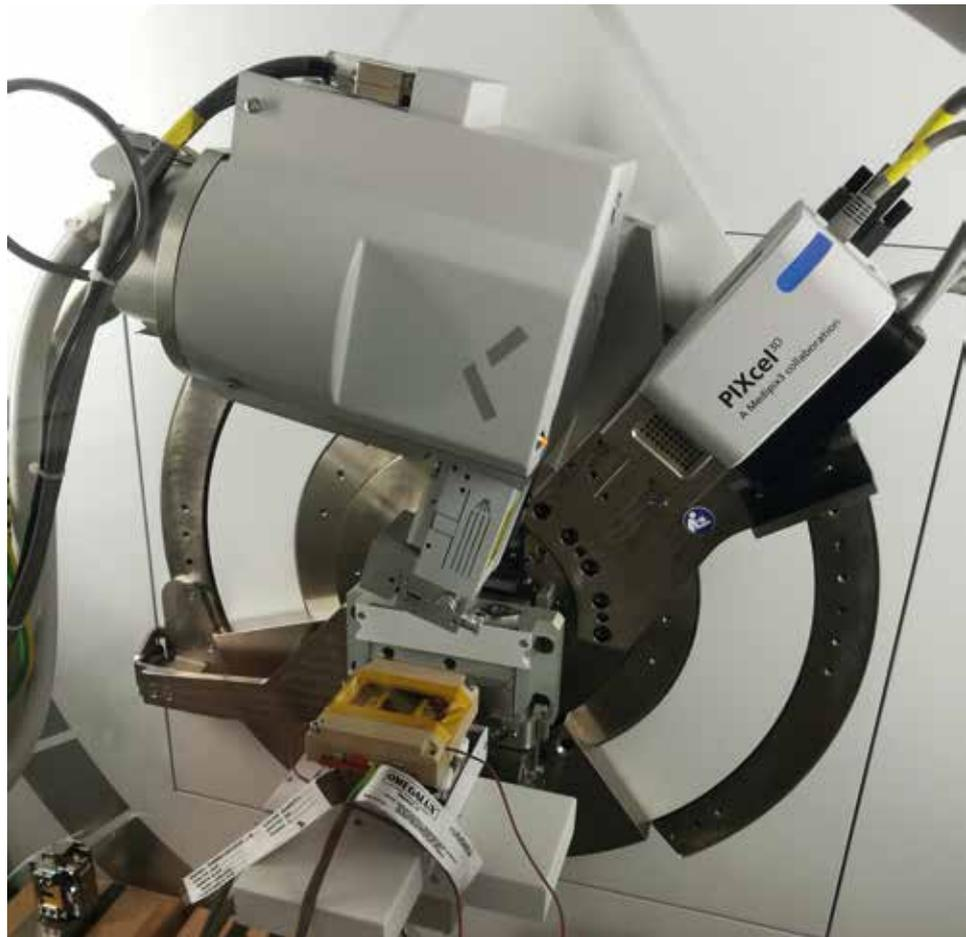
This equipment can be used to test the internal stress at different sample temperatures.
