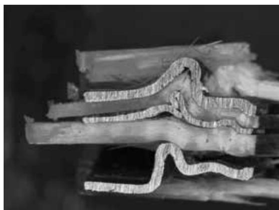
The situation that InHyb is trying to prevent: the bolt has deformed the metal sheet and damaged the GFRP material.
