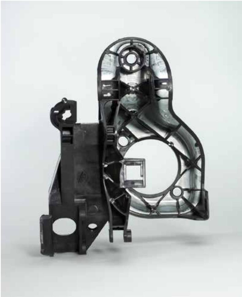
Pedal box made using hybrid technology: thin sheet profiles are reinforced with polyamide in the injection moulding tool.
